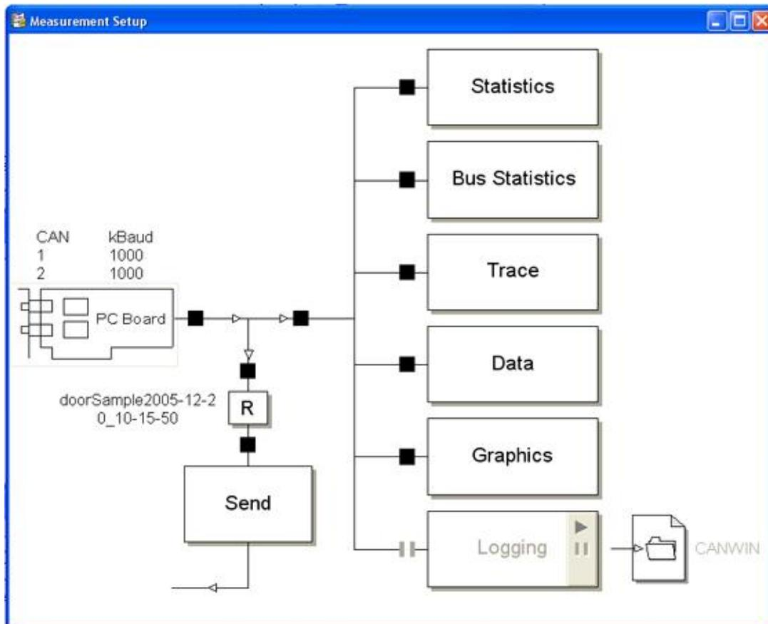
Figure 28. Measurement setup.
