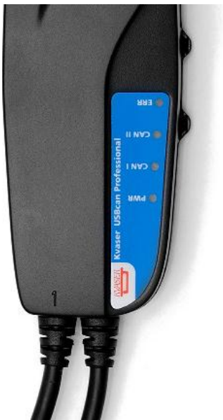
Figure 3: The CAN channels on Kvaser USBcan Professional.
