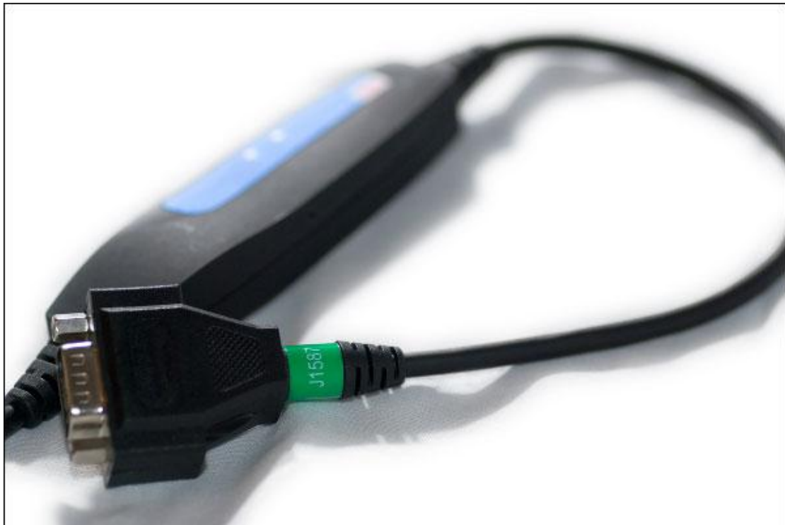
Figure 2: The J1587 connector on Kvaser Linx J1587.
