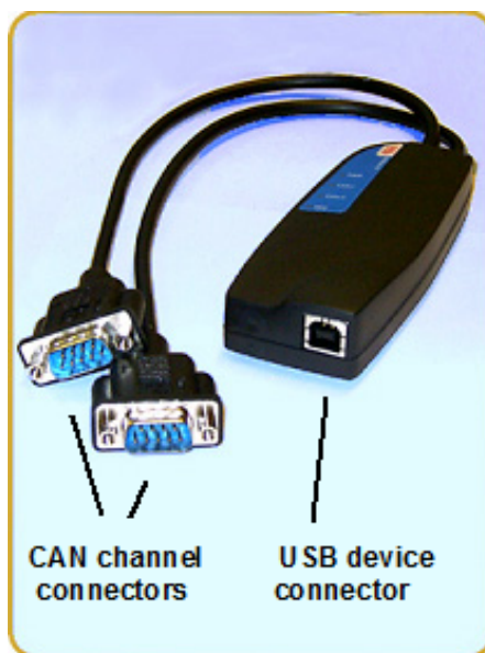
Figure 1: Connections on Kvaser Memorator
