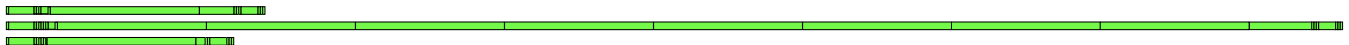
Figure 4, on top a Classical CAN frame with 8 bytes and in the middle a CAN FD frame with 64 byte with the same bit-rate. In bottom a CAN FD frame with 64 byte, but with bit-rate increased 8 times.
